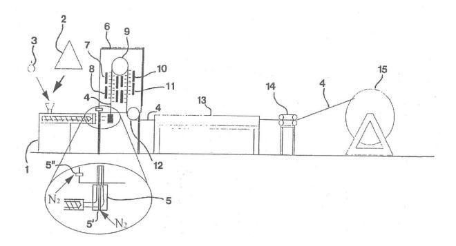
[26] The process, commencing at the left of the above diagram, is as follows: the peroxide (3) and polymer (2) are mixed in a hopper, and then enter the extruder. The extruded polymer pipe
